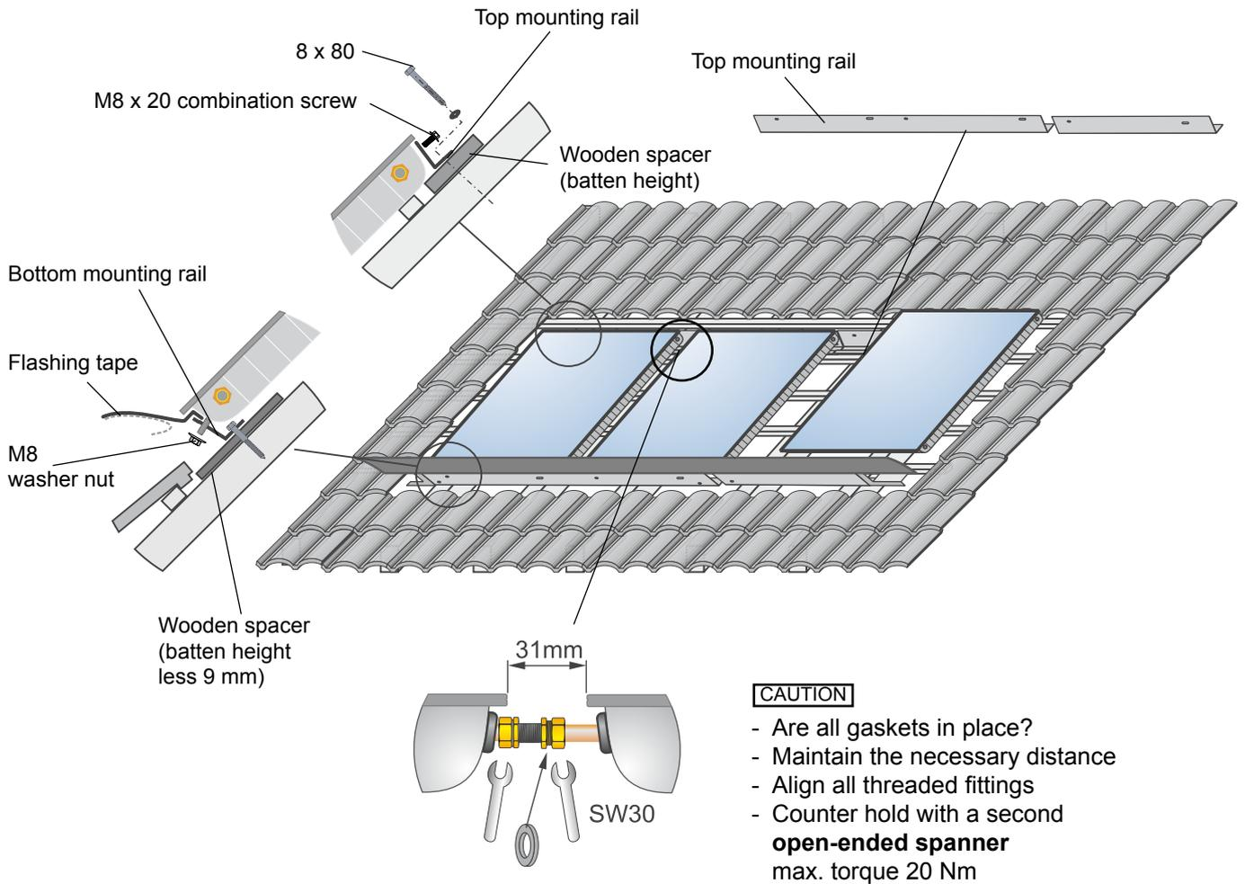
1. Insert the collector with the grub screws first into the lower mounting rail according to the diagram and initially secure it with the M8 nut with washer by hand.
