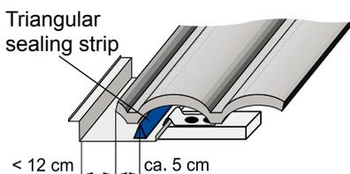
4. Affix the side and top triangular sealing strip to the casing panels.
