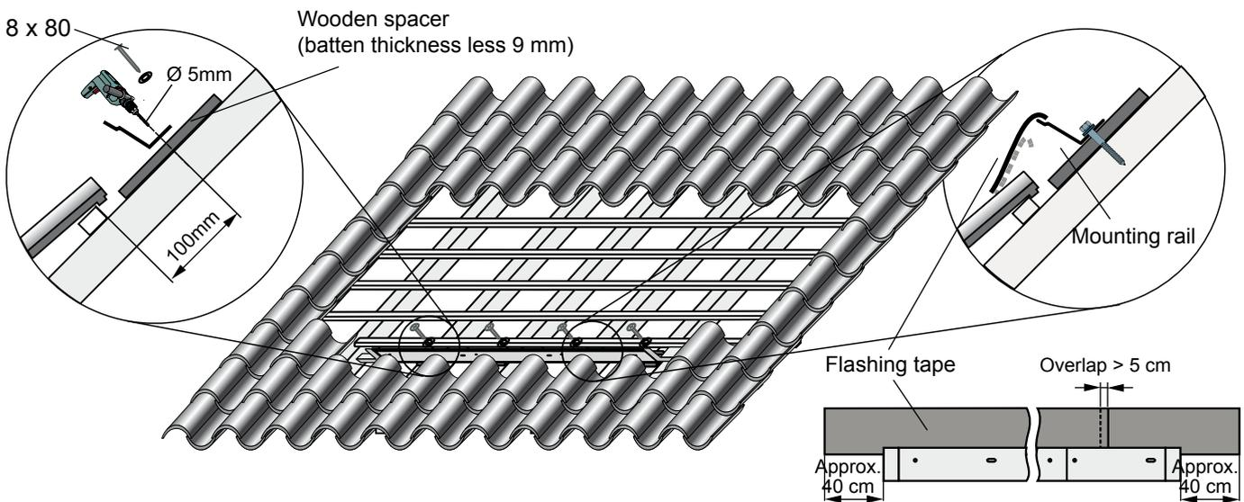
1. Pre-drill with  $\varnothing$  5 mm bit and secure the mounting rail and timber spacers (batten thickness less 9 mm) to the rafters with the hexagonal screws 8 x 80.
