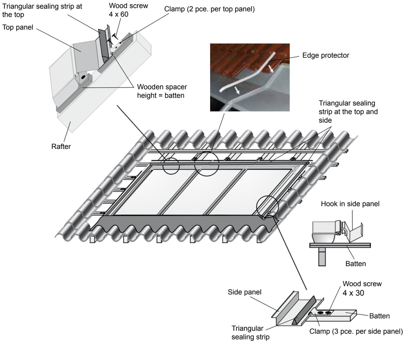
1. Hook in the casing panels on the left and right in accordance with the diagram and secure them with clamps.
