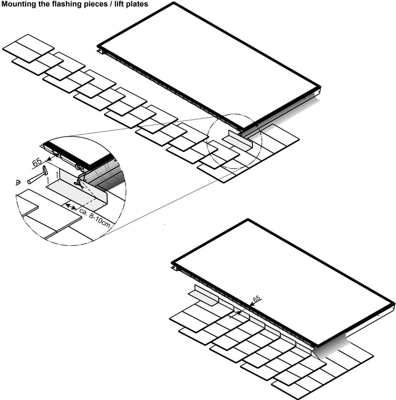
1. Fit bottom lift plate to the fold in the flashing tape and trim with scissors if necessary. Ensure sufficient overlap (8-10 cm).
