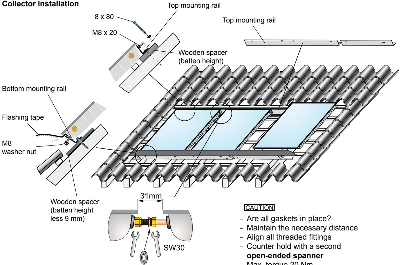
1. Insert the collector with the grub screws first into the lower mounting rail according to the diagram and initially secure it with the M8 nut with washer by hand.
