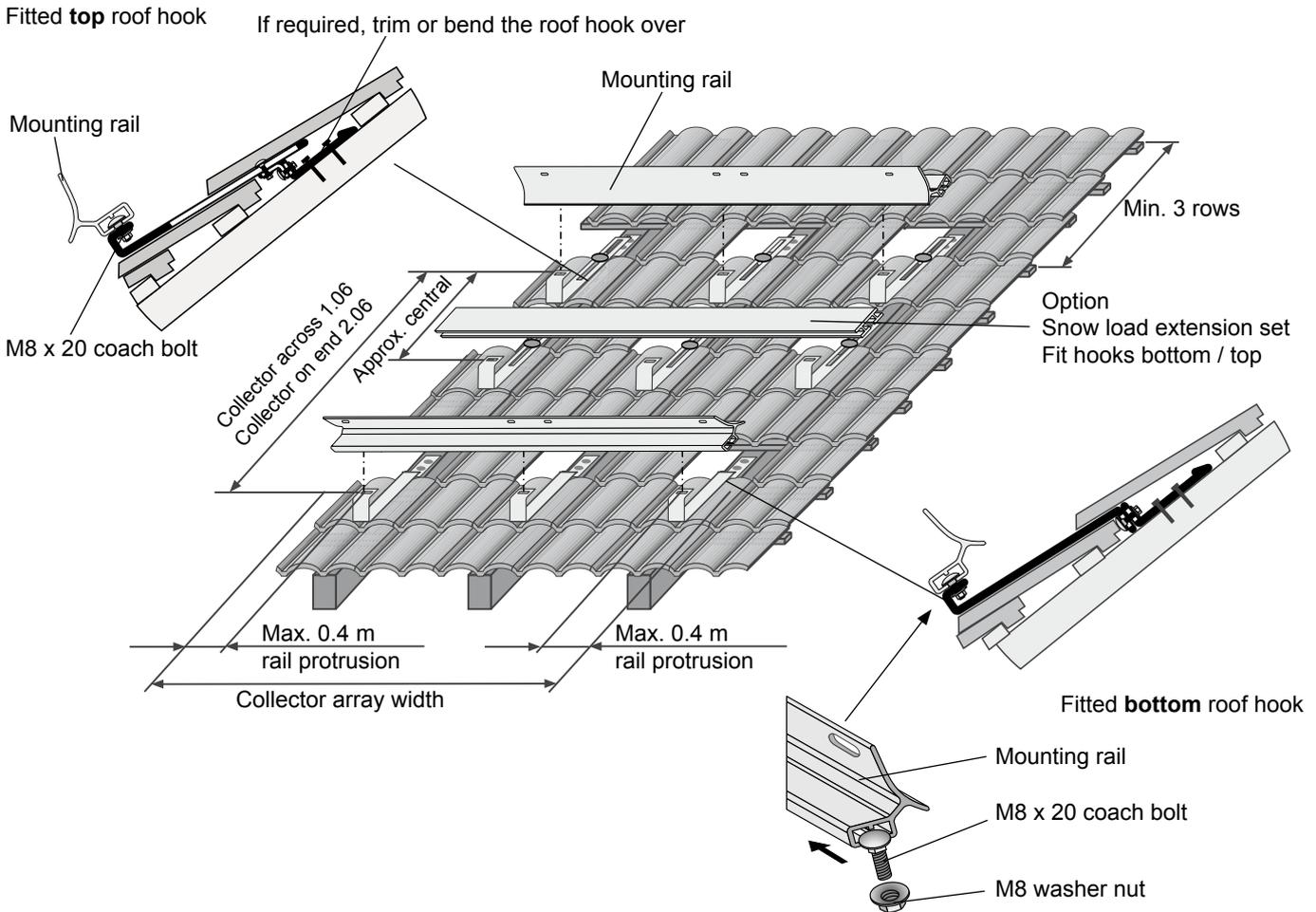
**CAUTION** Distribute all supplied double-ended screws evenly over the width of the collector array to spread the loads applied.
