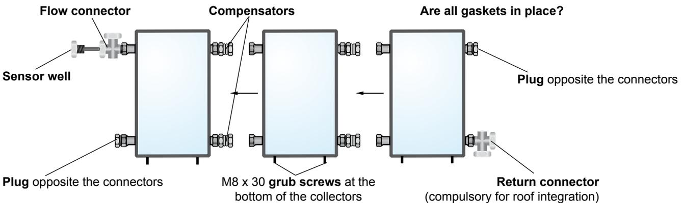
**Layout example: 3 F3-1Q / F3-Q collectors, across, single sided connection on the left (max. 5 collectors)**
