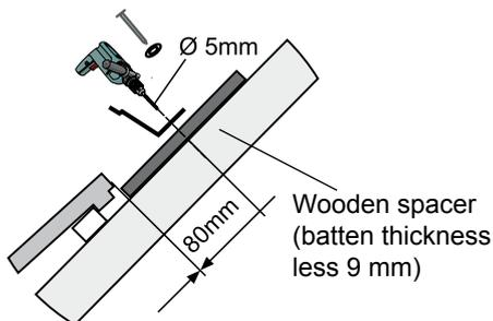
2. Drill a  $\text{Ø } 5 \text{ mm}$  hole and secure the mounting rail with the hexagon head cap wood screw 8 x 80 and the wooden spacers (batten thickness less 9 mm) to the rafters.
