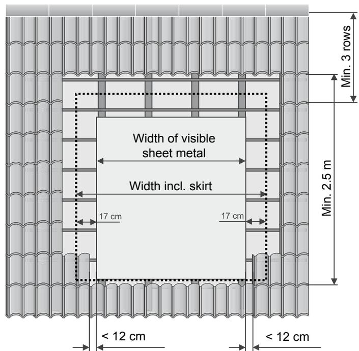
**Remove one extra row of tiles to provide sufficient space for installing.**
