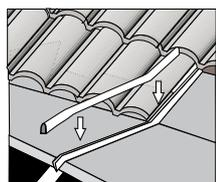
3. Push the protective edge profiles at the casing panel joint at the top over the return, see the diagram.
