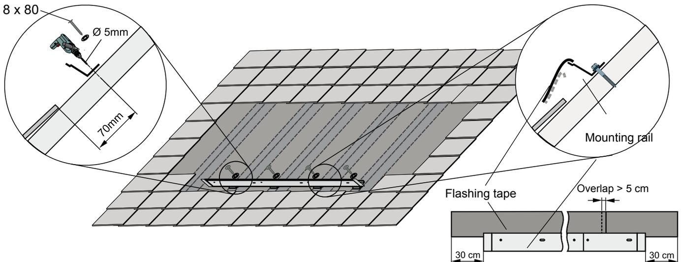
1. Pre-drill with  $\text{Ø } 5 \text{ mm}$  bit and secure the mounting rail to the rafters with the 8 x 80 hexagonal screws (provided).
