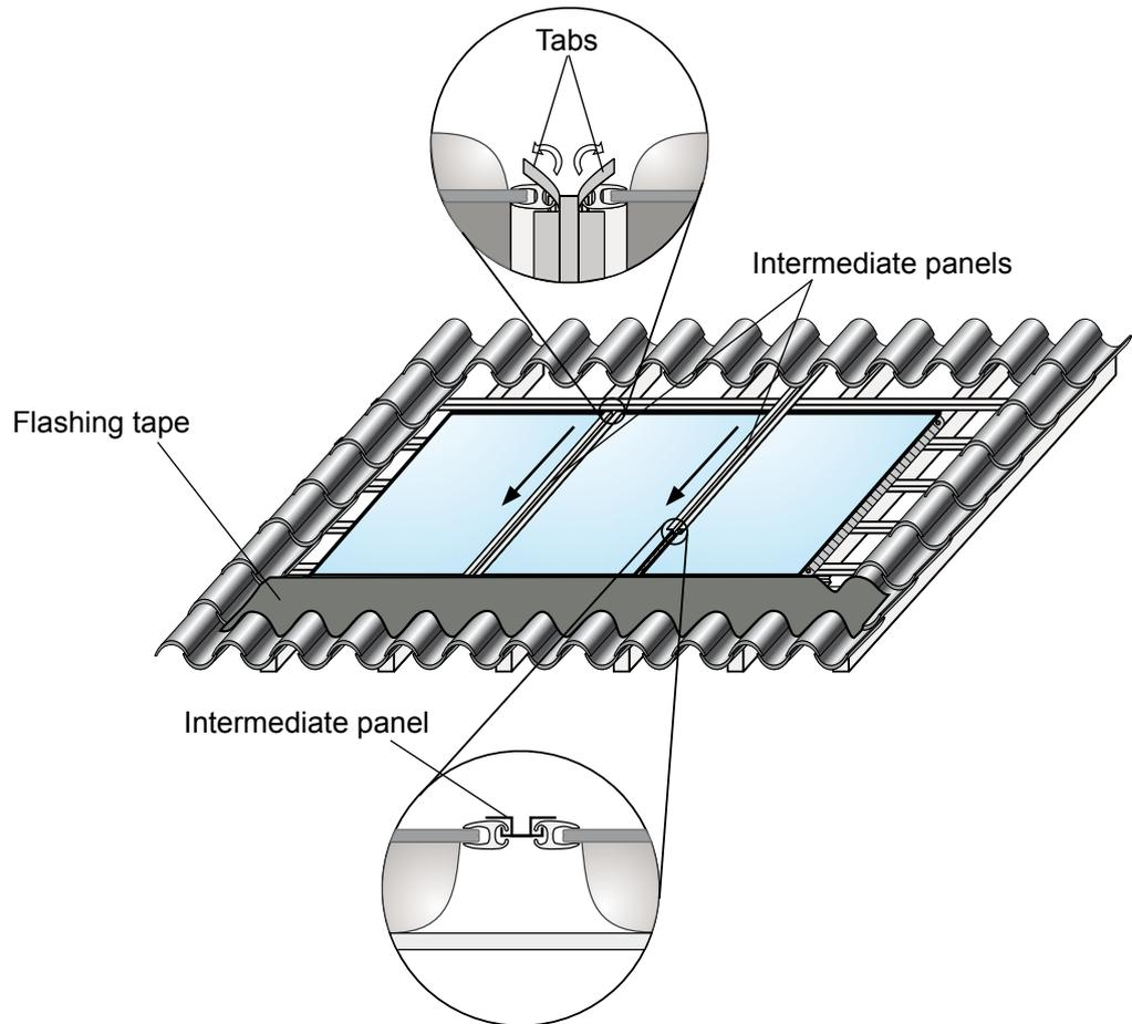
1. Push in the intermediate panels as per diagram. If this should foul during the installation, correct the collector position. Then bend the tabs at the top of the intermediate panels to prevent them from sliding through.
