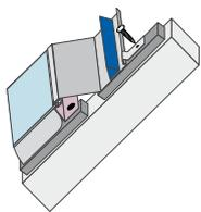
2. Push the top casing panels over the collector frame. As support on each rafter, a wooden spacer of batten height must be fitted below the casing panel. Secure the casing panel with clamps.
