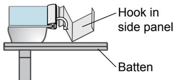
1. Hook in the casing panels on the left and right in accordance with the diagram and secure them with clamps.
