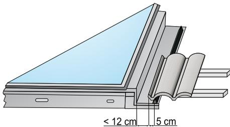
1. After fitting the extension, centre the mounting rail so that a gap of less than 12 cm is created on both sides between the collector array and the finished tiling. If this is not possible, use half tiles or cut tiles to size. Ensure that the gap dimension remains <12 cm to ensure the roof cover is fully rainproof.
