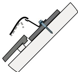
3. Affix the flashing tape in accordance with the diagram. For this, peel back the protective foil only in the area actually to be used for the mounting rail. The flashing tape must protrude approx. 30 cm on the left and right over the flashing tape bases. Secure several flashing tapes to each other with an overlap of at least 5 cm. (Do not as yet affix the flashing tape to the tiles as the collectors must still be secured to the mounting rail.)
