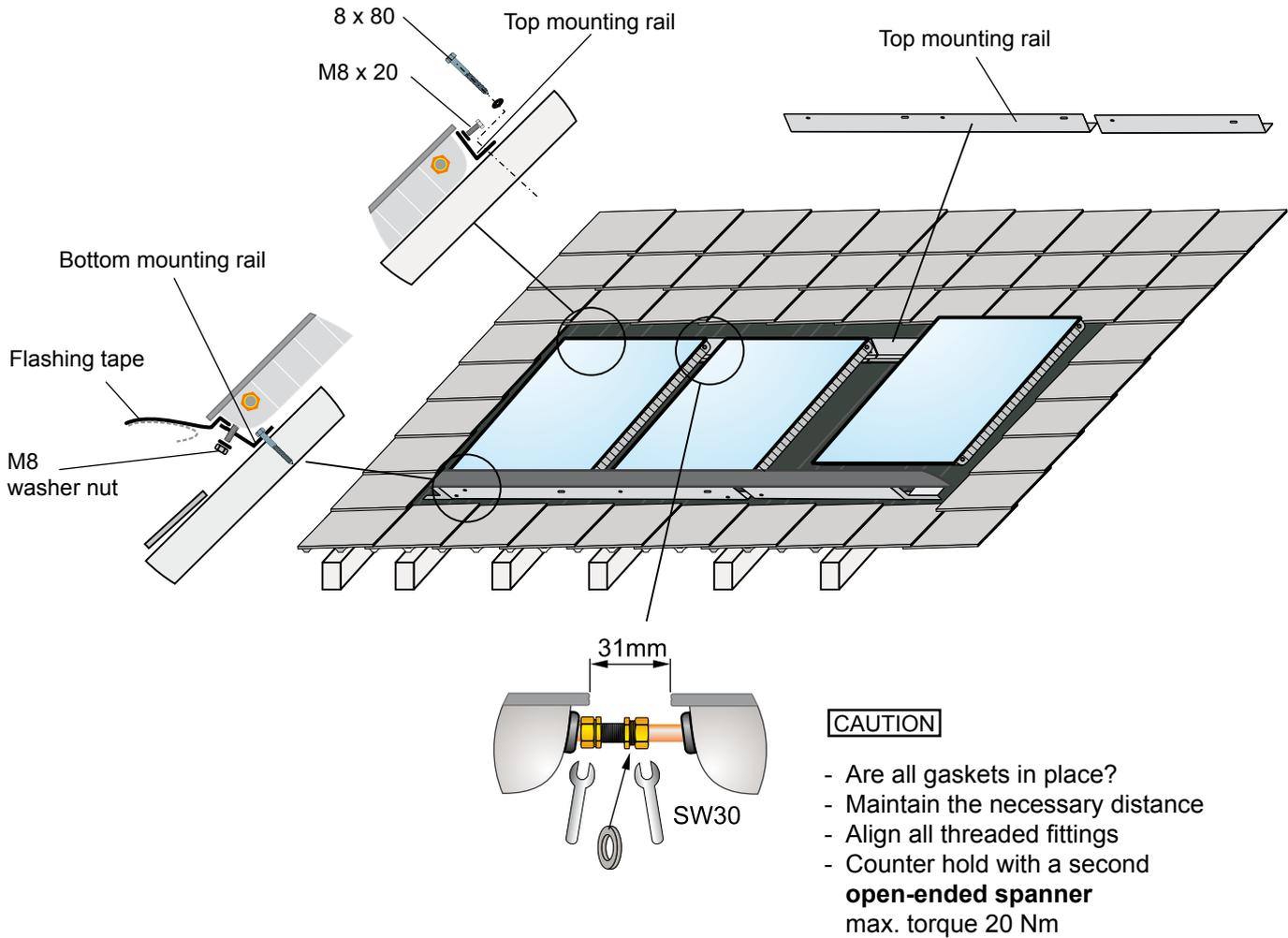
1. Insert the collector with the grub screws first into the lower mounting rail according to the diagram and initially secure it with the M8 nut with washer by hand.
