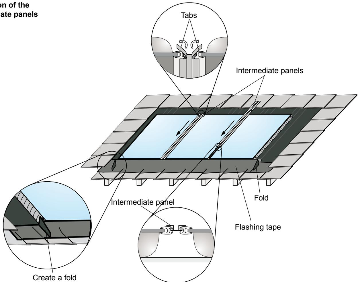
1. Push in the intermediate panels as per diagram. If this should foul during the installation, correct the collector position. Then bend the tabs at the top of the intermediate panels to prevent them from sliding through.
