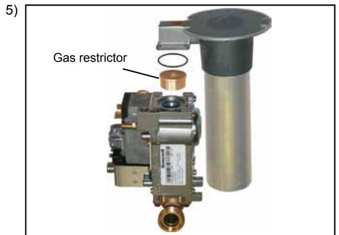
Remove integral gas restrictor and replace with the gas restrictor for the new gas type (in accordance with the table on page 25).
