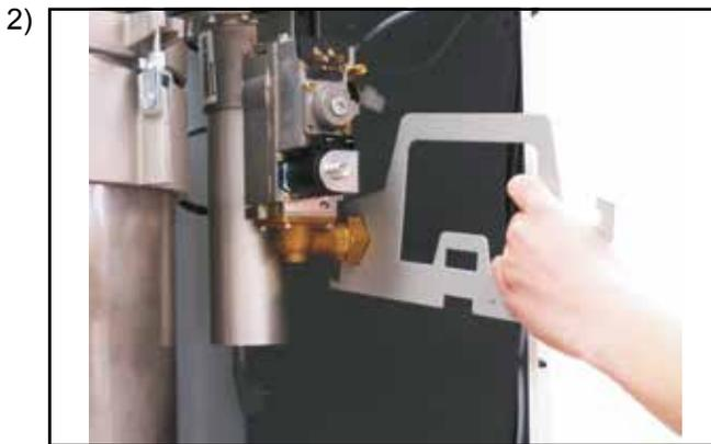
Undo gas connection at the gas combination valve
