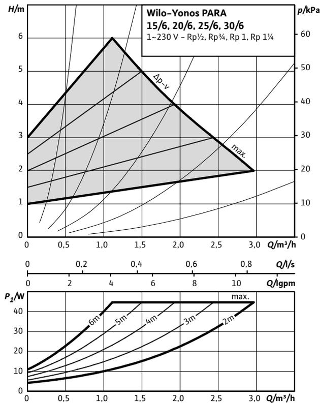
Tolerances of each curve according to EN 1151-1; 2006
