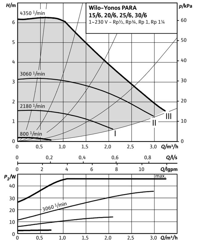
Tolerances of each curve according to EN 1151-1; 2006
