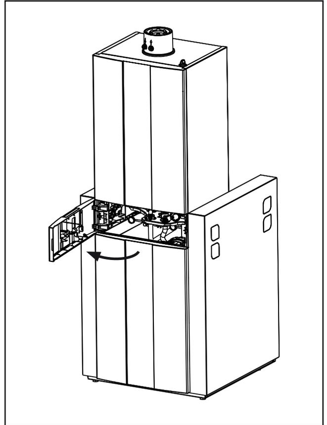
Fig.: Front view, control unit cover open
