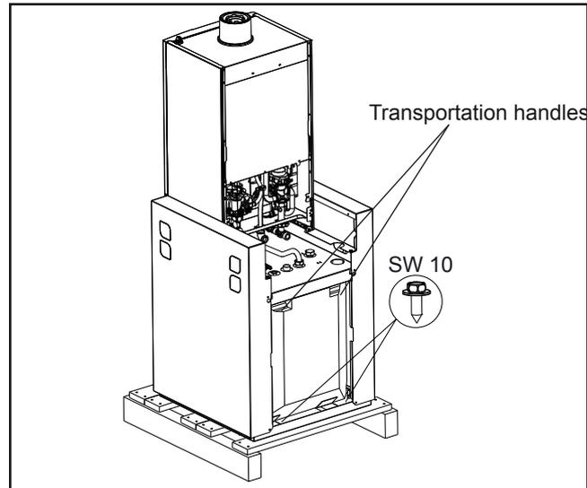
Fig.: Back transportation handles/locking screws
