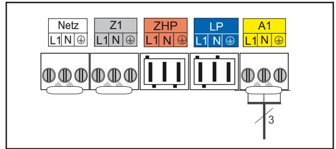
Fig.: Connecting output A1
