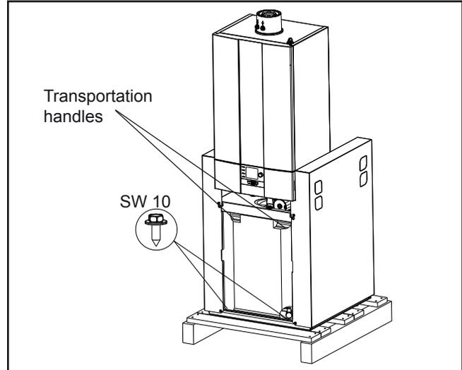
Fig.: Front transportation handles/locking screws
