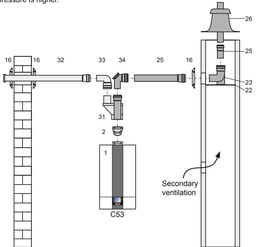
Maintain the following clearance between the flue and the internal duct wall:
