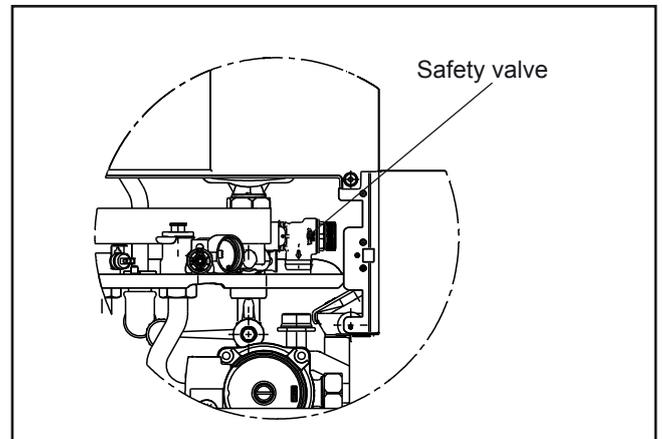
Fig.: Heating circuit safety valve (CGS-2L shown)
