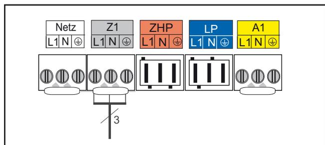
Fig.: Connecting output Z1
