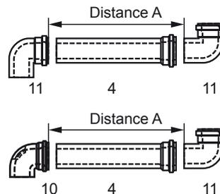
Determine distance A. Length of balanced flue (4) must always be approx. 100 mm longer than distance A. Always trim the flue on the smooth side, **never** on the female connection side.
