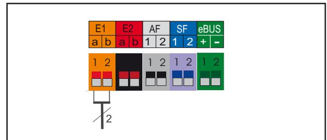
Fig.: Connecting input E1
