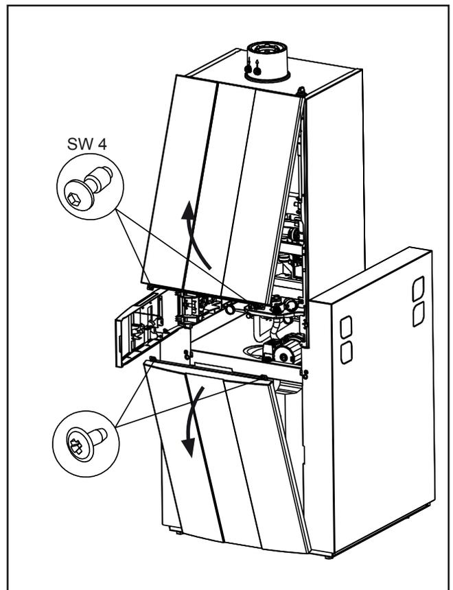
Fig.: Dismantling the stratification cylinder front casing
