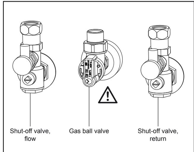
Fig.: Gas connection: Risk of poisoning or explosion in the event of gas escaping
