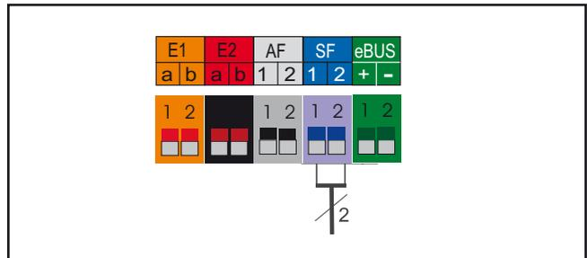
Fig.: Cylinder sensor connection
