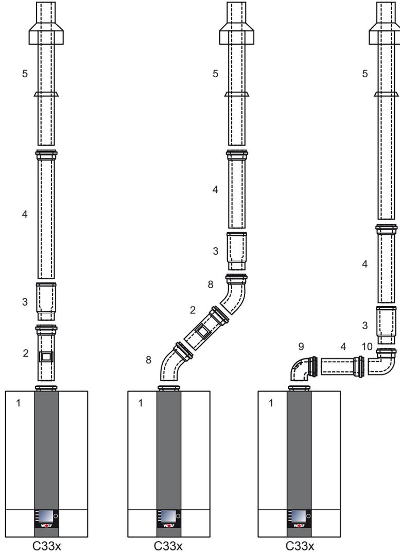
Installation examples for room sealed connections (vertical)
