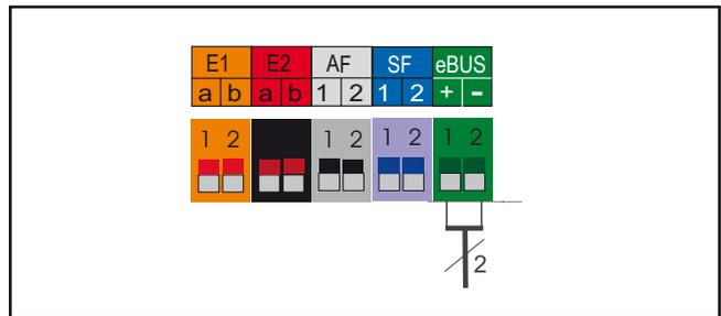
Fig.: Connecting digital Wolf control accessories (eBUS interface)
