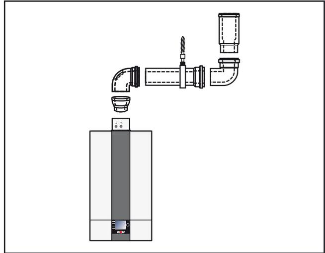
Fig.: Example: Balanced flue
