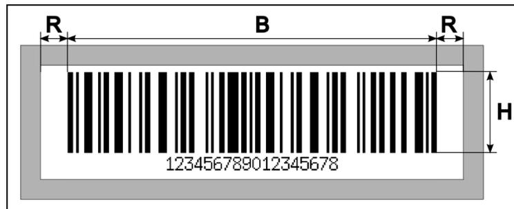
**Dimensions:** Based on the specifications above, the following minimum dimensions result for barcodes with the data structure types 1 - 4:
